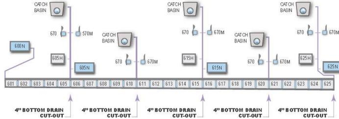
**NOTE 1:** All half and non-sloped channels have bottom cut outs.
