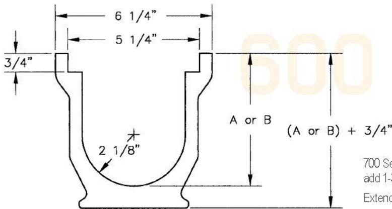
700 Series HARDNOSE and DURAGUARD® frames add 1-3/16" to dimensions A or B.
